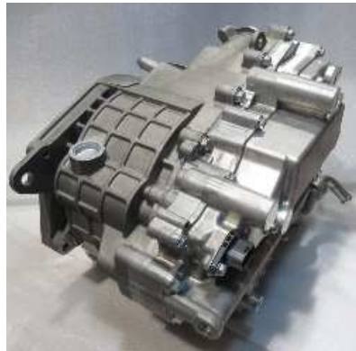
<Example : Integrated Motor/Inverter for EVs>
